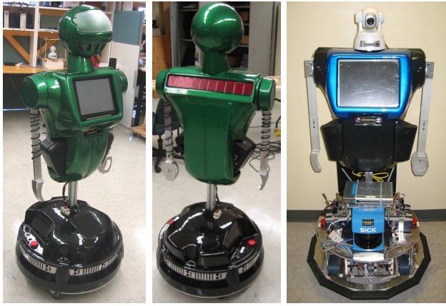
Fig. 1. U2S, the robot-ambassador of the Université de Sherbrooke, front view (left), back view (center) and Spartacus, the AAI version (right).
